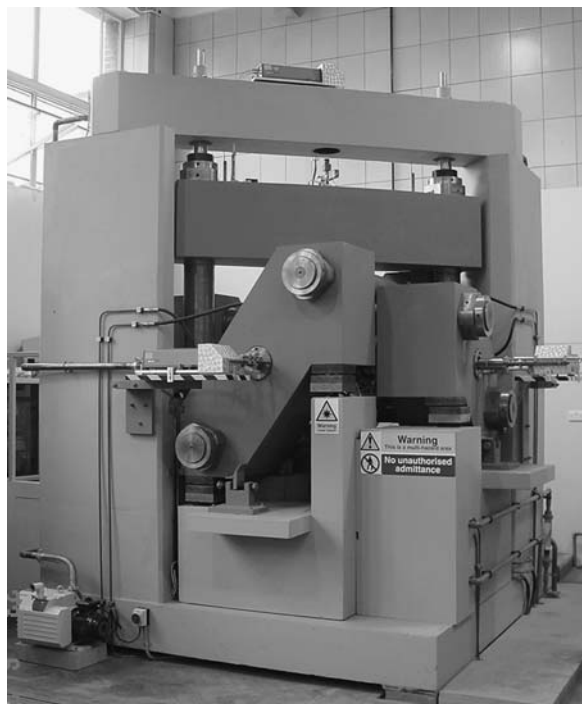
Fig. 1. mac^{2T} apparatus for multi-axial compression of concrete at elevated temperature
