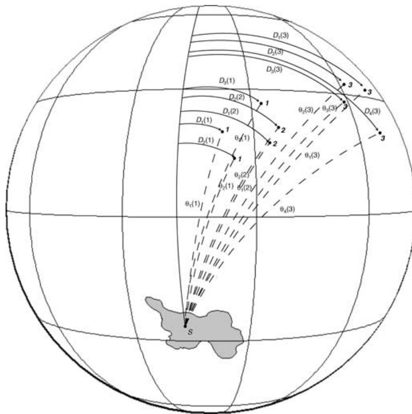
Figure 5. Sketch illustrating the role of declination, D_i , and colatitude, \theta_i , components of palaeopoles on the formation of APW paths. In this example three palaeopoles having comparable values of declination relative to a reference site S contribute for time 1, but the third of them has a bad colatitude component. This causes a shift toward the northeast of the mean palaeopole at time 1. Similarly, four palaeopoles having compatible values of the colatitude component contribute to the formation of a mean palaeopole for time 3. However, a bad declination value of the fourth of them determines a shift towards the southeast of the mean at time 3. Projection is a vertical perspective, with meridians and parallels equally spaced by 30^\circ .
