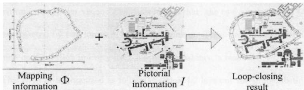
Figure 4.1: The loop-closing with appearance information.
