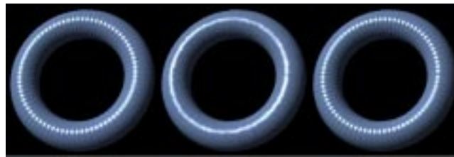
Figure 51: Bumpy Torus Model. Left: 44,252 triangles full resolution mesh. Middle and Right: 5,531 triangles, 0.25 mm maximum image deviation. Middle: per-vertex normals. Right: normal maps
