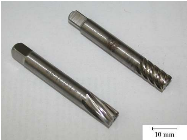
Fig. 4. Milling tools with 15° and 45° groove slope.
