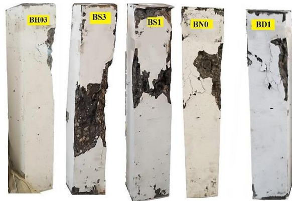
Fig. 12: The failure mode of uniaxial loaded column.
