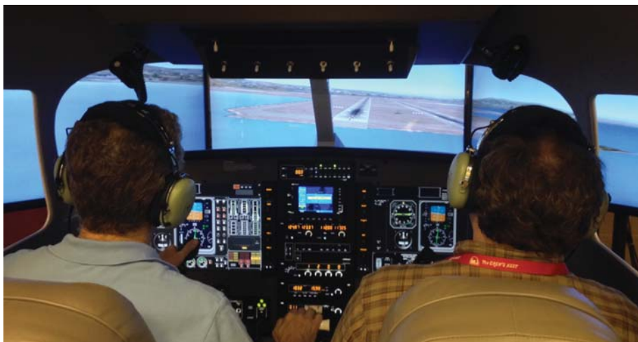
Figure 5. Interior view of flight simulation test bed for piloted evaluations.
