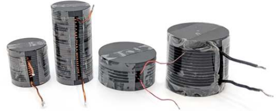
Fig. 9: Inductor prototypes with core configurations (left to right): MP17/1.0, MP17/2.0, MP27/0.5, MP27/1.0.
