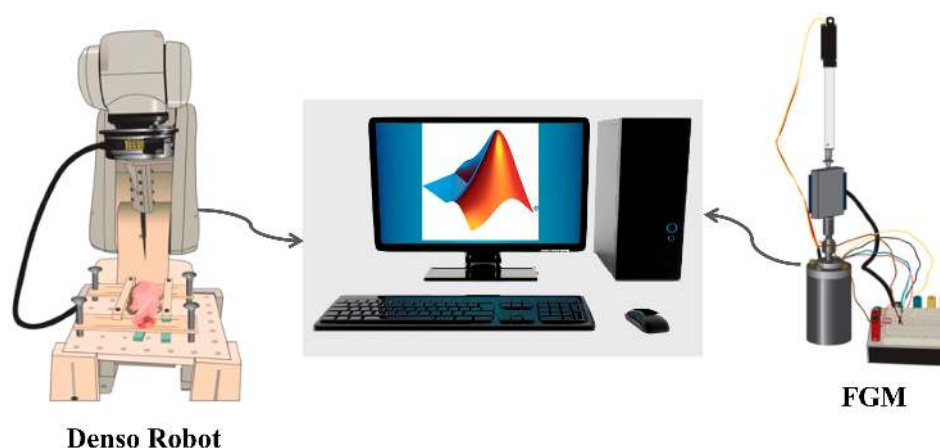
Figure 5. Experimental setup when connecting the FGM to the slave robot using a computer setting with MATLAB.
