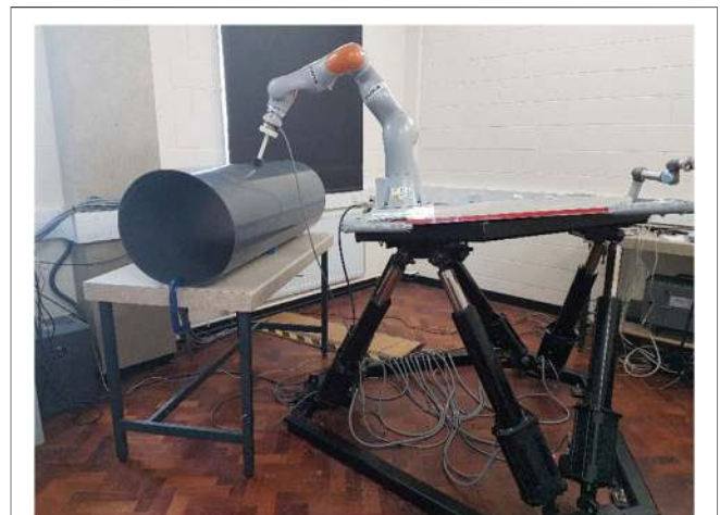
FIGURE 7 | Emulating UVMS via using a KUKA IIWA manipulator mounted on a Stewart Platform and interacting with a pipe.
