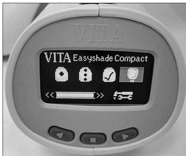
Figure 2. The device features: overall tooth shade determination, determination of the tooth shade for each third and verification of the shade of restoration
