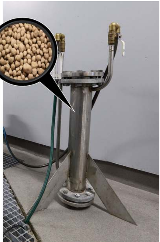
Fig. 2 Small pilot-scale set-up for ammonium removal from municipal wastewater using granulated metakaolin geopolymer (Luukkonen et al. 2017b). With this set-up, it was possible to reach < 4 mg/L \text{NH}_4^+ in cold wastewater ( \approx 10 °C)
