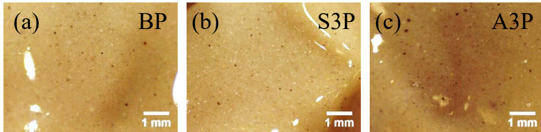
Figure 19: Surface images of filter cakes produced after the HPHT filtration (a) BP (b) S3P (c) A3P.
