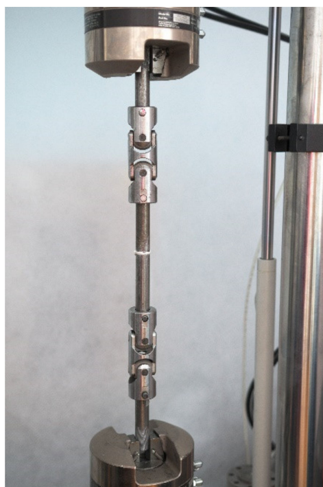
Figure 4. Fixtures with clamps (double-Cardan universal joint).
