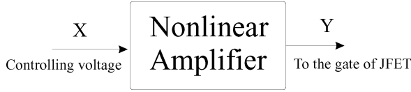
Fig. 8. Nonlinear amplifier which provides the gate voltage from V_C .
