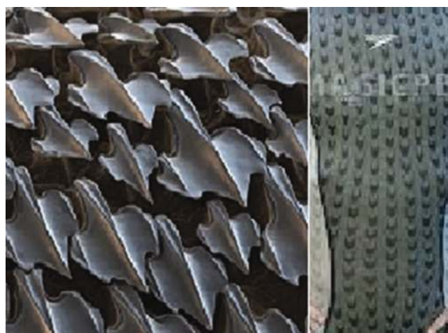
Figure 3. (Left) SEM of shark skin and (Right) Fastskin Fsii (FS2) swim suit, mimicking shark skin.
