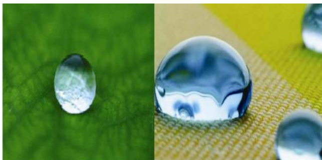
Figure 5. Lotus effect on the surface of a lotus leaf (left) and hydrophobic surface (right).
