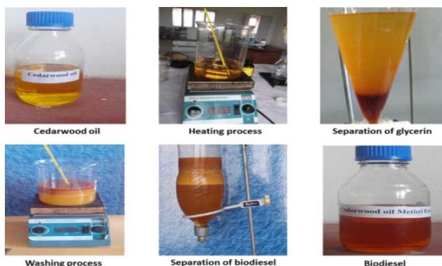
Fig. 1 Process involved during biodiesel production
