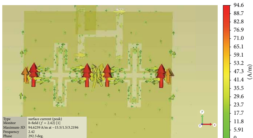
FIGURE 13: Current distribution in 3rd iteration fractal slot antenna with H-DGS.
