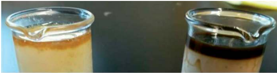
Figure 9. Filtrate from Jatropha oil-based emulsion (on left side) and filtrate from diesel oil-based emulsion (on right side) [56].
