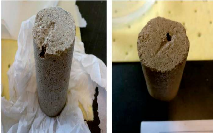
Figure 8. The cores used for investigating the diesel-based and Jatropha -based emulsified acids [56].
