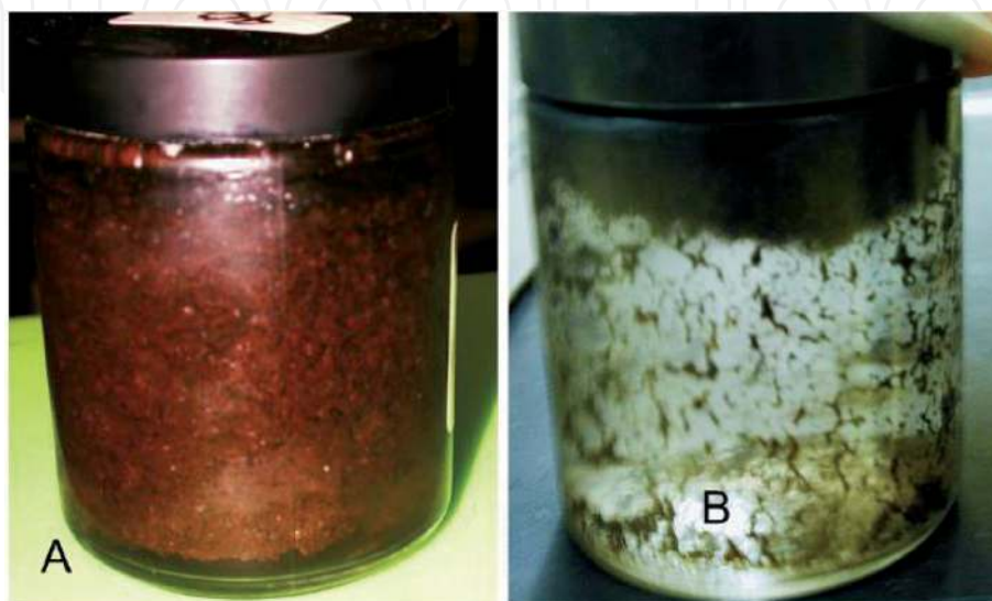
Figure 2. A photograph of stable emulsion (A) and unstable emulsion (B) [6].
