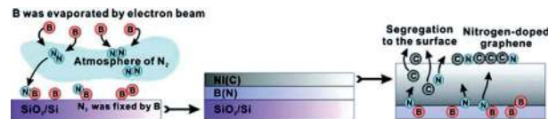
Fig. 1 Schematic diagram of the preparation of N-doped graphene. Reproduced from ref. 33 with permission from ACS, Copyright 2012.
