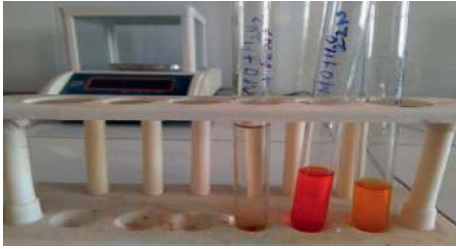
FIGURE 5: Dye degradation using iron nanoparticles.
