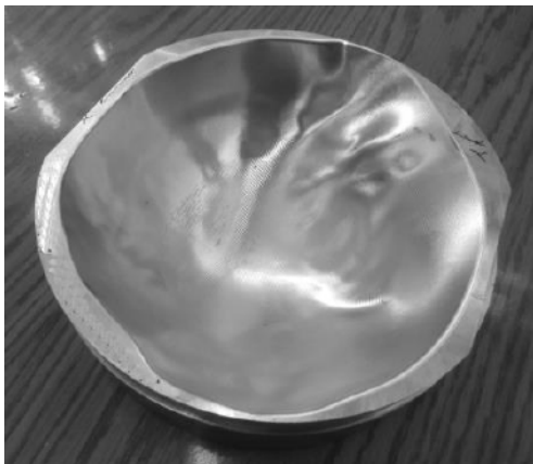
Fig. 7. Die-block for mould-incremental sheet forming.
