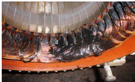
Fig. 7. Insulation damage occurred in 2010 in the same motor due to catastrophic failure of the bearings.
