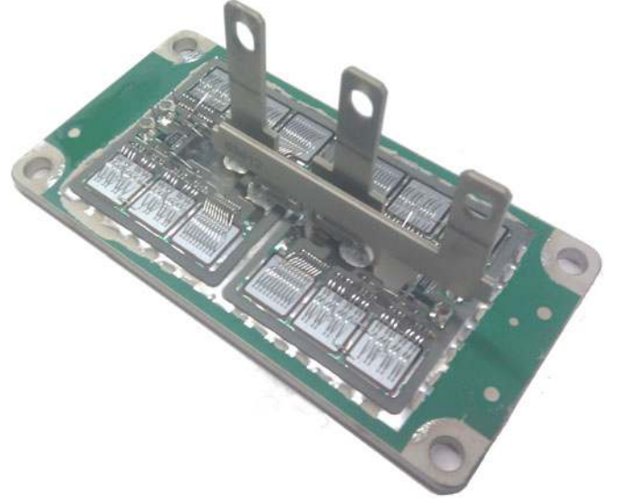
Fig. 6. 1.2-kV/400-A half-bridge power module used in the test. Each substrate tile contains four IGBTs and two freewheeling diodes.
