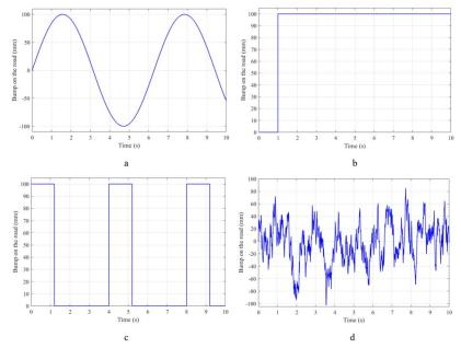
Figure 4: Bump on the road (a – Sine wave; b – Step; c – Pulse; d – Random).
