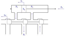
Figure 2: Hydraulic actuator.
