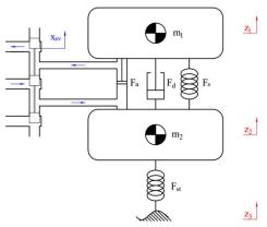
Figure 1: Model of the vehicle dynamics.
