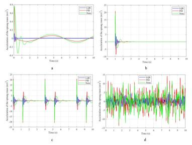
Figure 6: Acceleration of the sprung mass (a – Sine wave; b – Step; c – Pulse; d – Random).
