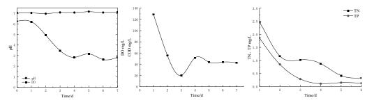
**Figure 4.** Variation in pH, DO, COD, TN, and TP of outlet water with time in the early stage of constructed wetland operation.
