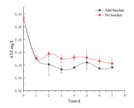
Figure 6. Changes in ATZ content in the outlet water with time.
