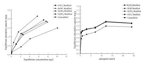
Figure 3. Adsorption isotherm curve (left) and adsorption kinetics curve (right).
