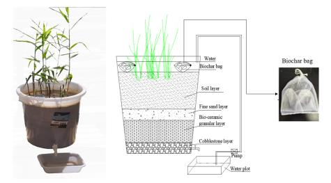
Figure 1. A schematic diagram of the simulated constructed wetland and the biochar bags.
