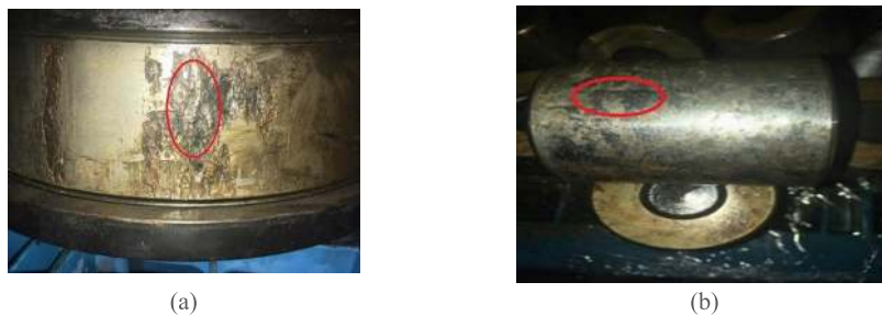
FIGURE 7. Bearing inner ring and rolling element failure diagram. (a) Bearing inner ring peeling off; (b) bearing rolling body pitting.
