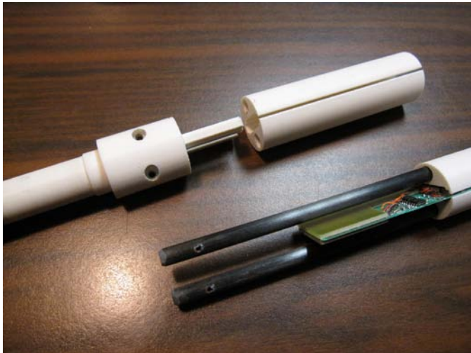
Fig. 6. A 24mm PCB probe supported within an FDM fabricated structure with carbon-fiber rods.
