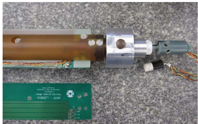
Fig. 5. Strong-back support of PCB probe which allows for different width circuit boards to be tested.
