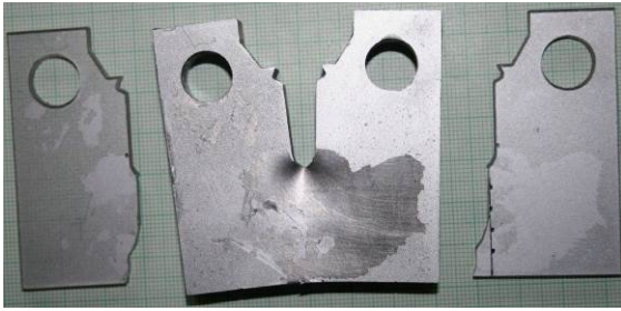
Figure 15. Damaged photoelastic coating PS-1A with the notched sample and relative elongation 4%
