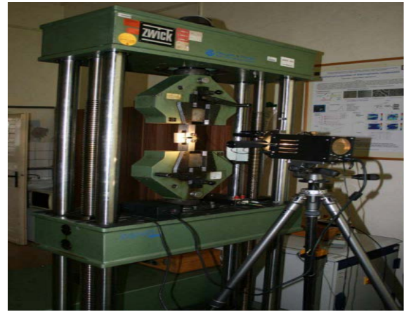
Figure 3. Tearing machine Zwick 1387 with reflection polariscope LF/Z-2
