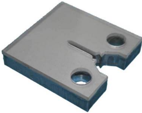
Figure 2. Analysed sample with photoelastic coating PS-1A
