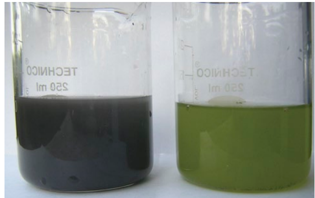
Figure 3 Photograph showing the dissolved ETP solid before and after phycoremediation. Before treatment, the dissolved ETP solid, which was black in colour, turned to green due to rich algal growth.
