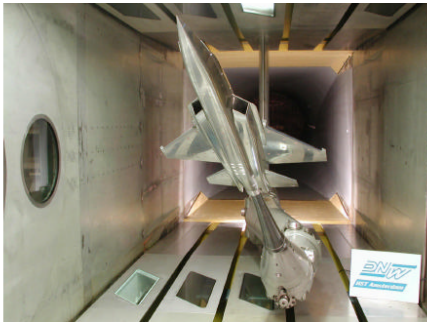
Fig. 7. Model in the test section of the DNW-HST wind tunnel
