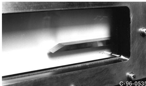
Figure 4.—Oblique shock wave generator.
