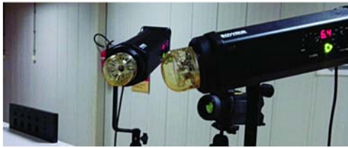
Figure 2. Flash pulsed thermography system
