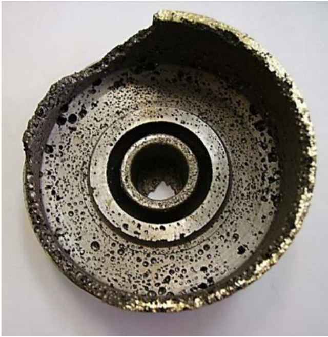
Fig. 3. Typical defects of the submersible pump guide vanes formed during casting: pores and caverns.
