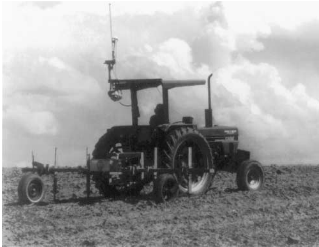
Fig. 7. Mobile fixed-array equipment for the continuous measurement of apparent soil electrical conductivity.
