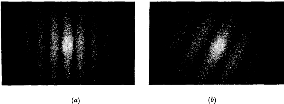
Figure 6. Photographs of the cosine fringes in the Fourier plane of the doubly exposed speckle pattern obtained with stroboscopic illumination of the tuning fork. (a) 2|\Delta\xi| = 19 \mu\text{m} , (b) 2|\Delta\xi| = 13.4 \mu\text{m} .
