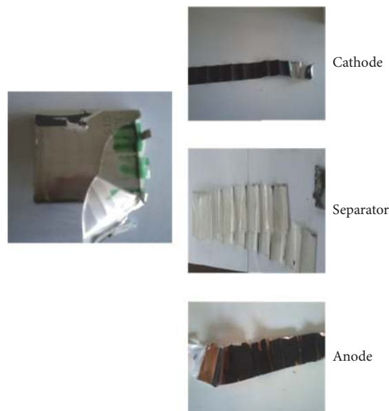
FIGURE 2: Cathode, anode, and separator from a cell phone spent LIB used in this work.
