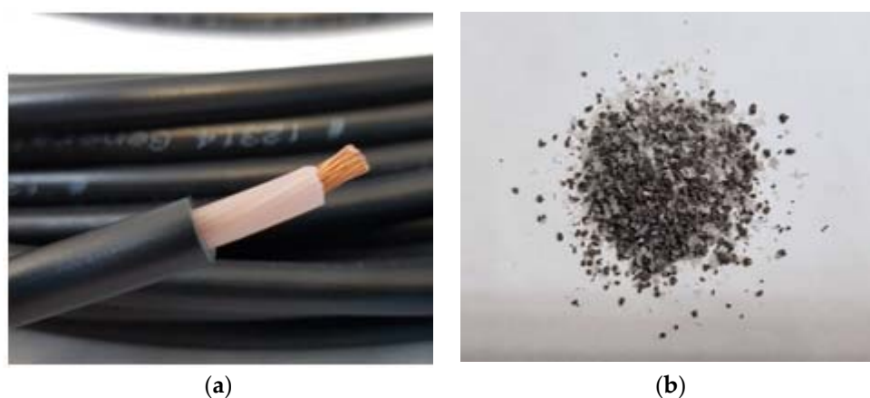
Figure 1. Electric wire used in the runs (a) before crushing process; (b) after crushing process.
