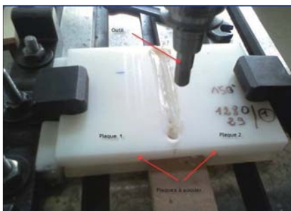
Fig. 1. Butt weld of HDPE thick sheet.
