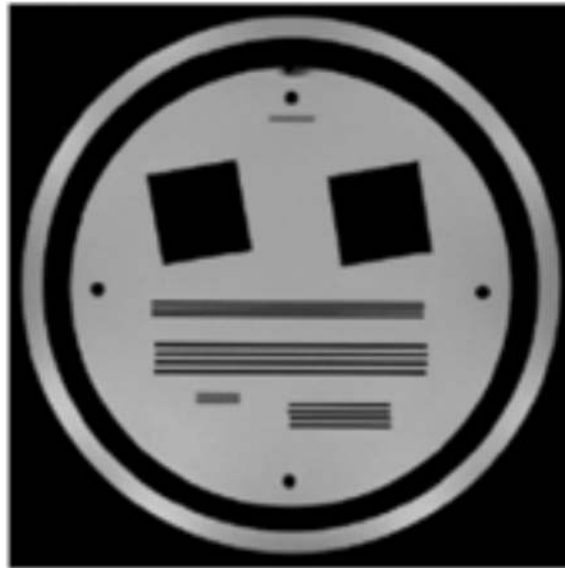
Figure 3 An MR image of the Eurospin TO4 test object which allows the assessment of image spatial resolution.
