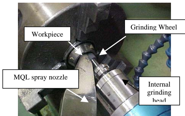
Figure 1. Position of the MQL spray nozzle in the cutting region.
