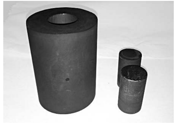
Fig. 3. The graphite die used to bond the copper rods, with the two 20 mm-diameter pressing cylinders.
