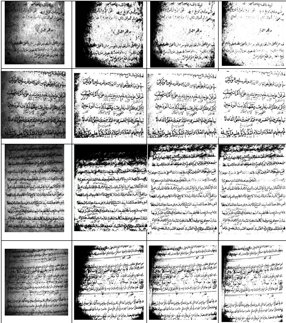
Figure 6: (a) Image before binarization (b) Result of Otsu's method (c) Result of Niblack's Algorithm (d) Result of Sauvola's Algorithm
