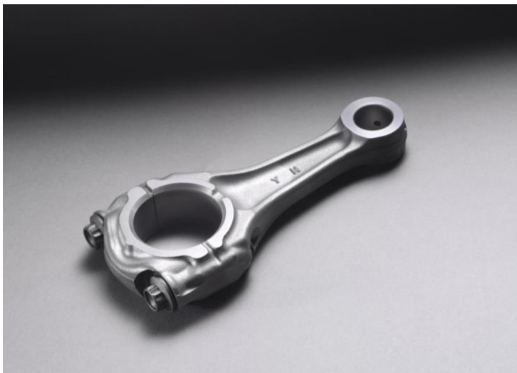
Figure 5. Appearance of the fracture-split connecting rod made of Ti-5Al-1Fe.
