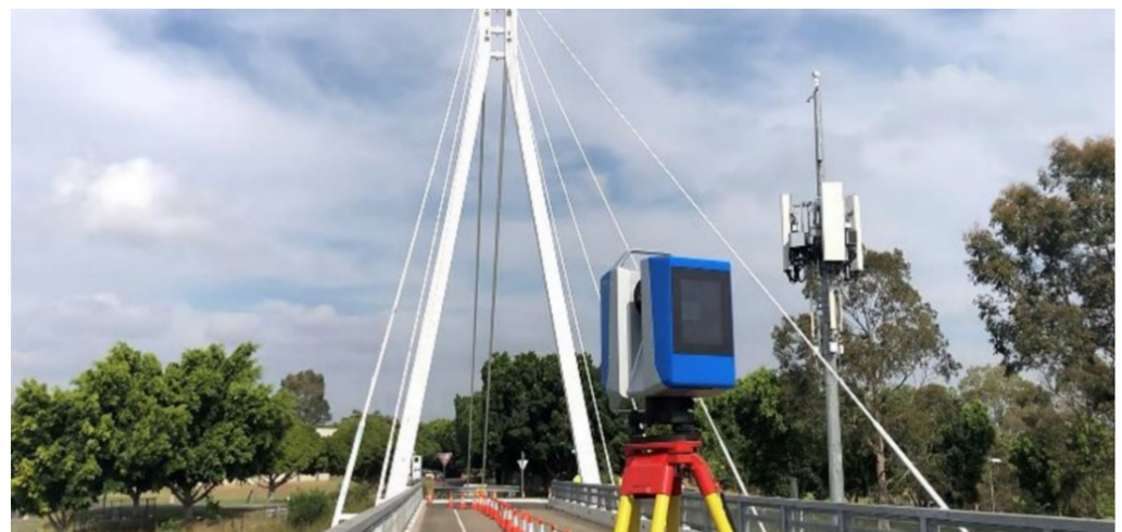
Figure 5. Laser scanning of Werrington bridge.
