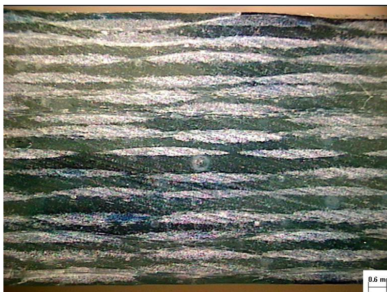
Fig. 8. Cross section ( \times 100 ) of GFRP specimen showing the elliptic shape of the fiber yarns
