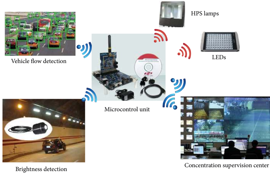
FIGURE 3: The tunnel illumination intelligent control system network structure.
