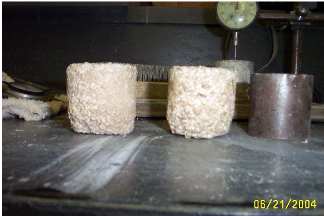
Figure 57: Specimens after Freeze/Thaw Tests (Left and Center); Steel Cylinder Control Volume (right)
