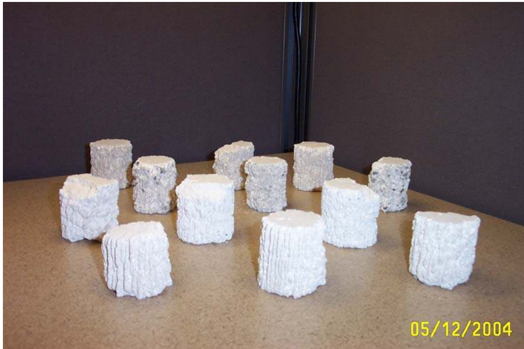
Figure 56: Wet/Dry Durability Test Specimens, after 12 cycles with Brushing
