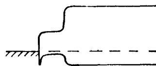
FIG. 13. — Generalized band-scheme for contacting a larger bandgap compound with a smaller bandgap compound. (Possible potential spikes are neglected here.)
