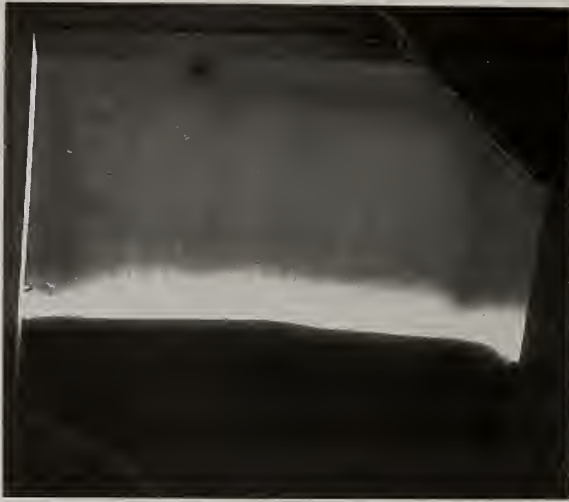
Figure 1. A scanning electron micrograph (x20) of a 4 x 4 mm C(100) diamond after electrochemical treatment. The IC (hydrogenated) is on top, the IA (oxidized) is below, separated from the IC by the "stripe" transition region.
