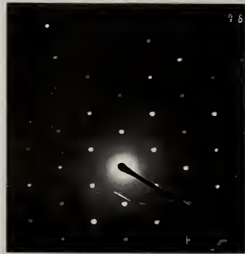
Fig. 3b Diffraction pattern from C:N film (T=180 °C).
