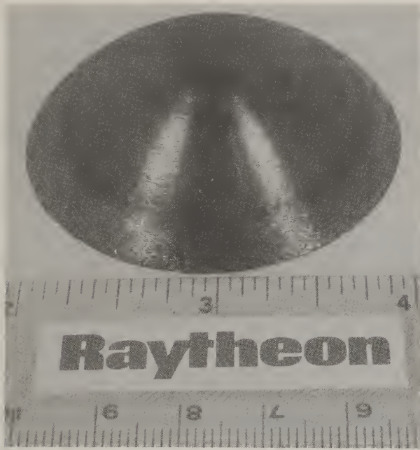
Fig. 3. Diamond dome that has been machined to hemispheric shape with a laser.
