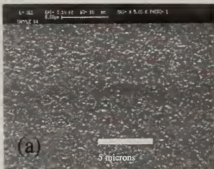
Figure 3. Scanning electron micrographs of (a) the growth surface of a membrane, facing the glass in the 'flip' configuration; and (b) the nucleation side of the membrane, facing away from the glass support in the 'flip' configuration.
