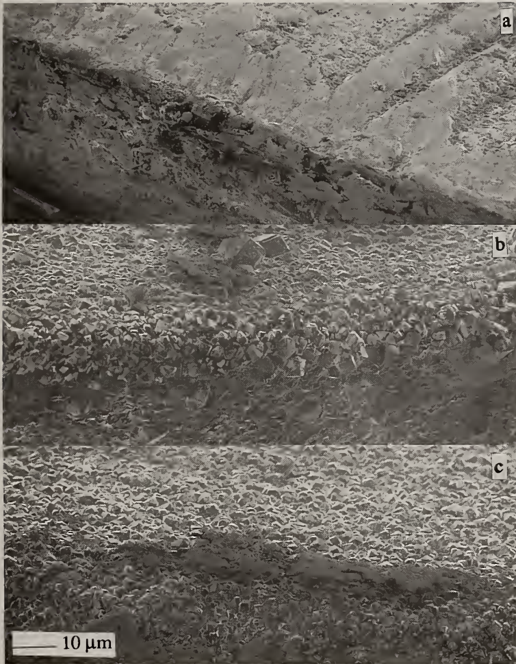
Fig. 4 SEM photographs of wear surfaces of WC tool (a), WC tool coated with single layer of diamond (b), and WC tool coated multilayer diamond (c) after dry fly cutting.
