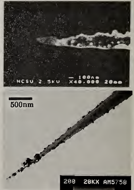
Fig. 2. Electron micrographs of c-D and a-D coated Si tips.
