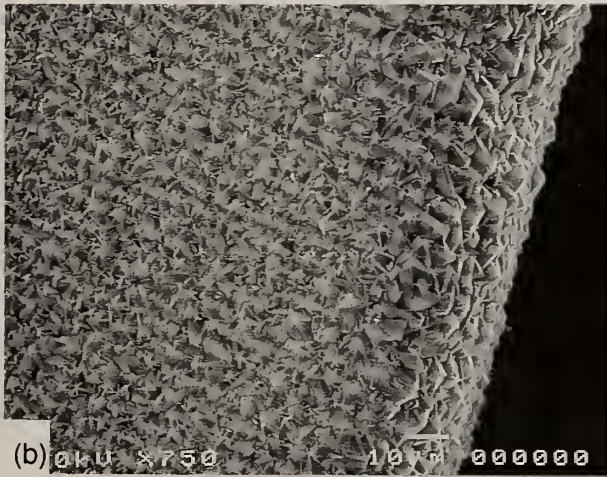
Fig.6. Scanning electron micrographs of diamond-coated end mills after cutting tests with A390 : (a) The arrows indicate workpiece, (b) Enlarged view of edge after washing with acid, showing no wear.
