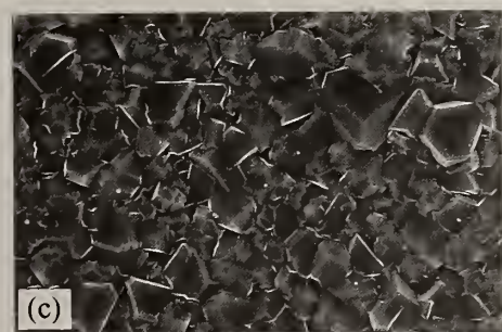
Fig. 2 SEM photographs of diamond films at radius distance of 10-15 mm when rotational speeds are (a) 0, (b) 1000 and (c) 2000 rpm
