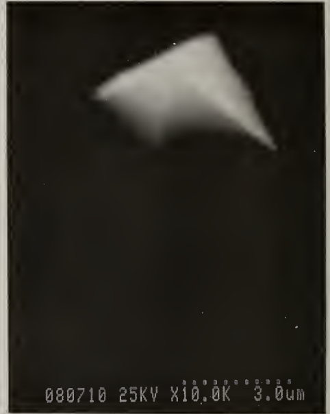
Fig. 2 A single pyramidal microtip on diamond.
