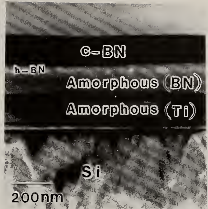
Fig. 4 Cross-sectional transmission electron micrograph of the c-BN film.
