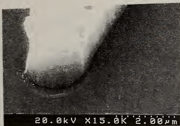
Fig. 3 SEM micrograph of a single crystal diamond after etching in high mode plasma
